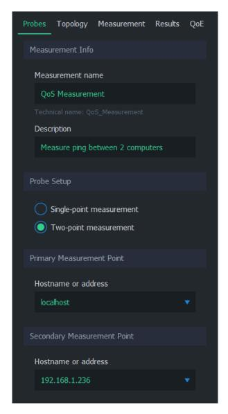
That's all for Probe setup. Having a two-point measurement will require some additional setup in measurement configuration, which is explained in the next sections.
