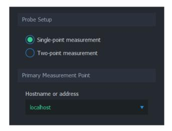
The location where the selected Probe is installed is called the **Primary Measurement Point**. The *Hostname or address* of this location can be given as a hostname or as a plain IP address, for example node.domain.com or 192.168.1.3.
