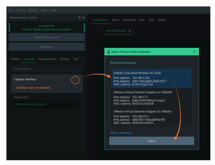
We'll select the network card which is connected to the Internet from the dropdown list by double-clicking, or clicking it once and then pressing **Select**. In this computer, that interface would be *Intel(R) Dual Band Wireless-AC 8265*.
