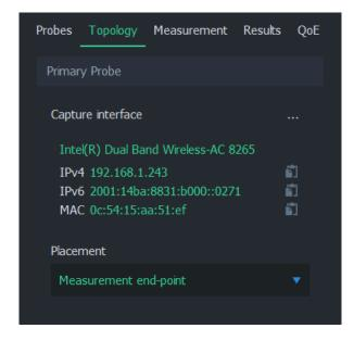
Next, we need to tell Qosium something about the network topology in order to help it determine the direction of the traffic. In a single-point measurement, we only need to inform Scope the placement of the Probe in relation to the measurement path. The options are:
