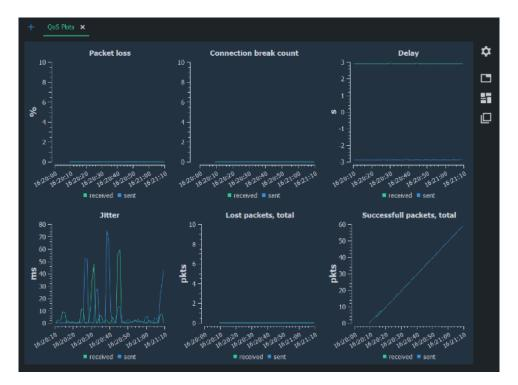
The plots already give lots of information about our test environment: The traffic has no lost packets, but there seems to be a large jitter variation. In the delay plot, we see an interesting result that delay seems to be negative to one direction and about similarly positive to the other. This is caused by clock synchronization error between the two measurement computers. See <a href="Time Synchronization">Time Synchronization</a> for more details and how to solve it.
