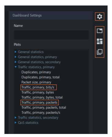
From the Plots list, select two result types: *Traffic, primary, bits/s* and *Traffic, primary, packets*. Two plots will appear immediately, displaying the traffic load in terms of bits and packets moving between this computer and the Internet. You can reorder and rearrange plots by using the buttons below the gear icon.
