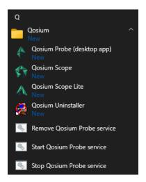
Use *Qosium Probe* (desktop app) to launch Probe in a command prompt window. Alternatively, select *Start Qosium Probe* service to set the Probe as an active Windows service. In that way, Qosium Probe is always in the background and starts with your device. To stop it, select *Stop Qosium Probe service*. To remove it from the Windows' service list, select *Remove Qosium Probe service*.
